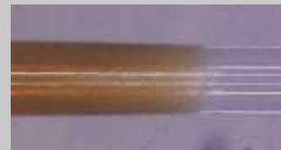
Polyimide stripping: Polymicro 330/300 μm, Polyimide coating shown.
