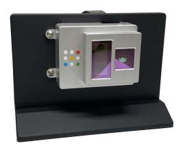
Experience the advantages of solid-state, software-defined lidar powered by LCM beam steering with the **M30 Evaluation Kit**, which includes:
