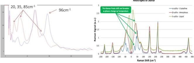
Ondax's patented<sup>2</sup> THz-Raman<sup>®</sup> Spectroscopy Systems extend the range of traditional Raman spectroscopy into the terahertz/lowfrequency regime, exploring the same range of energy transitions as terahertz spectroscopy - without limiting the ability to measure the fingerprint region. This enables simultaneous analysis of both molecular structure and chemical composition for advanced materials characterization.
