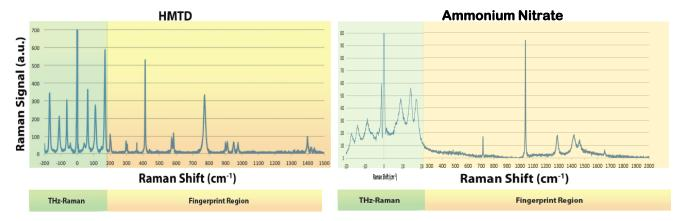
Ondax's patented THz-Raman® Spectroscopy Systems extend the range of traditional Raman spectroscopy into the terahertz/lowfrequency regime, exploring the same range of energy transitions as terahertz spectroscopy – without limiting the ability to measure the fingerprint region. This enables simultaneous analysis of both molecular structure and chemical composition for advanced materials characterization.
