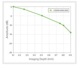
The Cobra VIS uses proprietary optics and a high sensitivity camera to deliver better roll-off than most OCT spectrometers, improving your resolution at increasing depths.
