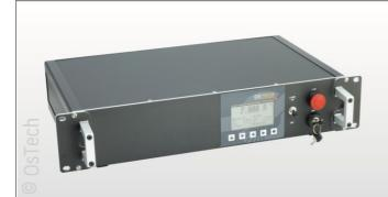
The product series ds11-t192 of table top drivers has all features of the ds-series. It is powered by an input voltage of  $110^{\sim}230$ VAC with power factor correction. The power ranges up to 1500W. The laser diode current ranges up to 120A and voltage up to 48V.
