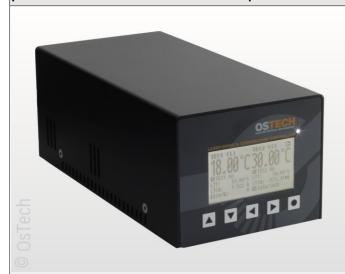
The product series ps11-t95 of table top drivers has all features of the ds-series. It is powered by an input voltage of 110~230VAC with power factor correction. The power ranges from 100W to 600W. The TEC current ranges up to 20A and voltage up to 48V.
