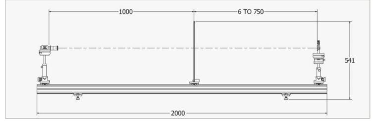
Dimensional drawing of BP100 side view with P501 imaging photometer. Dimensions are in mm.
