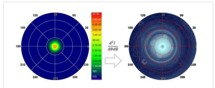
High current, 25 mm LED lamp / reflector assembly with clear lens, log-pseudocolor mapped.  $\Theta$  grid lines are at  $10^{\circ}$  intervals.
