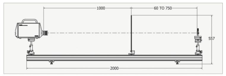
Dimensional drawing of BP100 side view with WP214 colorimeter. Dimensions are in mm.
