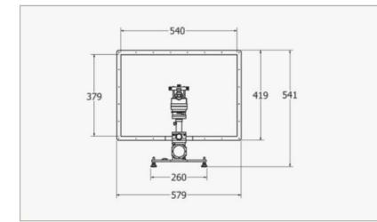
Dimensional drawing of BP100, end view. Dimensions are in mm.
