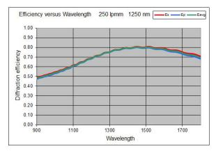
We offer broadband grating designs with highly efficient, low polarization-dependence performance at bandwidths of up to 1000 nm in the VIS/NIR, as modeled here.
